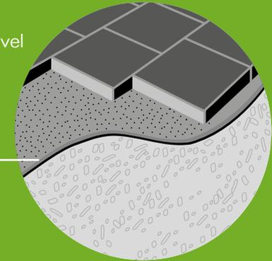
Lay GROUNDTEX Woven Geo Fabric beneath the sub-base to form a stable and level patio area.
