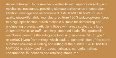
EARTHWORX NW1000 can also be used as a drainage and separation layer in the construction of horse arenas, subject to the joints being
